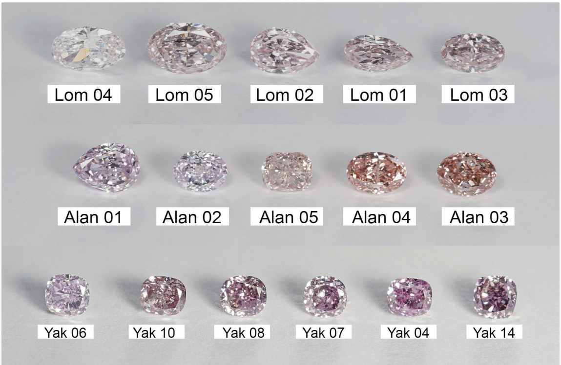
Fig. 2 Pink and purple diamond samples used for this study: Lomonosov mine, Severalmaz (upper row), Alan, Anabar (middle row), and Yakutia (bottom row). Size range is from 0.16 ct to 0.50 ct. Colour grades: from Faint Pink to Fancy Vivid Pinkish Purple. FOV 45 mm. Photo by Ioanna Kirillina.
